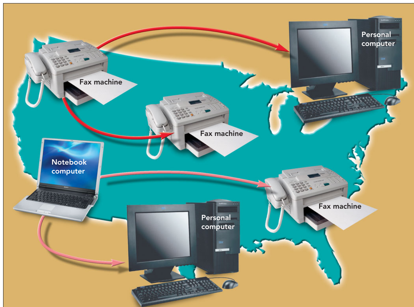
FIGURE 8.40 Facsimile transmissions can be sent over telephone lines or the Internet through the use of fax machines or computers equipped with fax modems.
