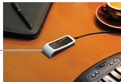
FIGURE 3.21 Biometric input devices use retinal scans to match the shape and pattern of an individual's eye and fingerprint readers to detect the shape, curve, and unique pattern of lines on a finger.
