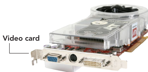
FIGURE 2.16 Expansion cards enable you to enhance and customize your system to meet your own personal needs.
