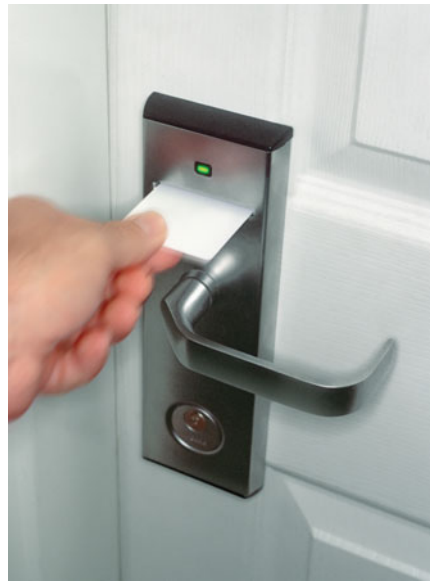
FIGURE 3.47 Smart cards can be used for quick transactions, to identify the user, or to access electronically controlled doors.
