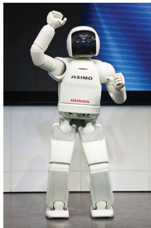
FIGURE 1.35 Asimo is a humanoid robot that stands 4 feet 3 inches and weighs 114 pounds. It can walk and run on two feet at rates of up to 4.3 miles per hour.
