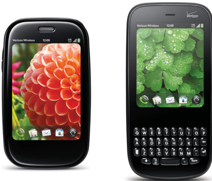
FIGURE 4.30 The Palm webOS, used on mobile devices like the Palm Pixi, offers quick access icons for e-mail and contacts along with a full set of menus to set preferences and access photos and text messages.
