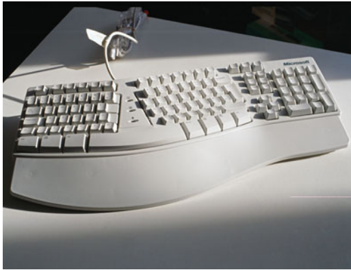
FIGURE 3.10 Ergonomic keyboards usually have a raised surface, a wrist rest, and a key display split down the middle.
