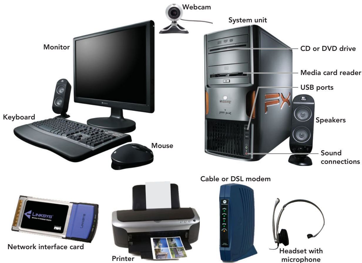
FIGURE 1.6 Get to know your system. A typical computer system includes these hardware components.
