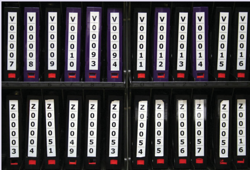
FIGURE 1E A backup system can help protect a business's information assets and enable the business to continue to operate as usual. A computer tape library is one way to store backed-up files.
