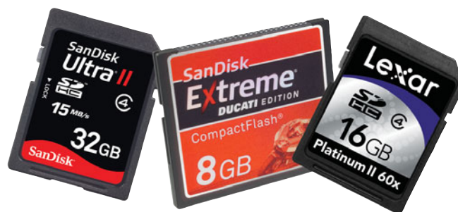
FIGURE 3.45 Flash memory cards are thin, portable solid-state storage systems.
