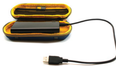
FIGURE 1.11 Hard drives can store very large quantities of data, making them the media of choice for activities that generate large files like movies, pictures, and backups.
