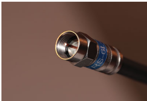
FIGURE 8.10 In coaxial cable, data travels through the center copper wire core. The cable is connected to a coaxial wall jack.
