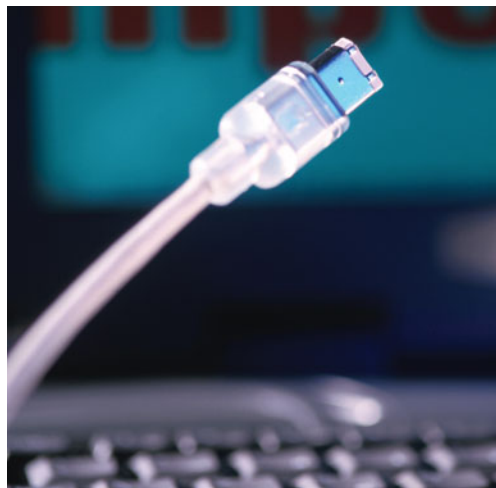
FIGURE 2.32 FireWire cables are used with FireWire ports to transmit digital video or audio files at high rates of speed.
