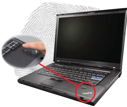
FIGURE 2.13 This fingerprint reader is one of several devices that provide biometric authentication.
