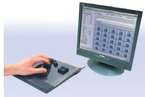
FIGURE 3.9 The Ergodex DX1 is revolutionizing input systems by allowing individuals to customize the location and function of input keys.
