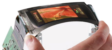
FIGURE 3.28 This flexible OLED communication device is worn on the wrist and was developed in conjunction with the U.S. Department of Defense.
