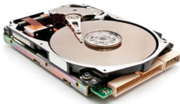
FIGURE 1.11 Hard drives can store very large quantities of data, making them the media of choice for activities that generate large files like movies, pictures, and backups.
