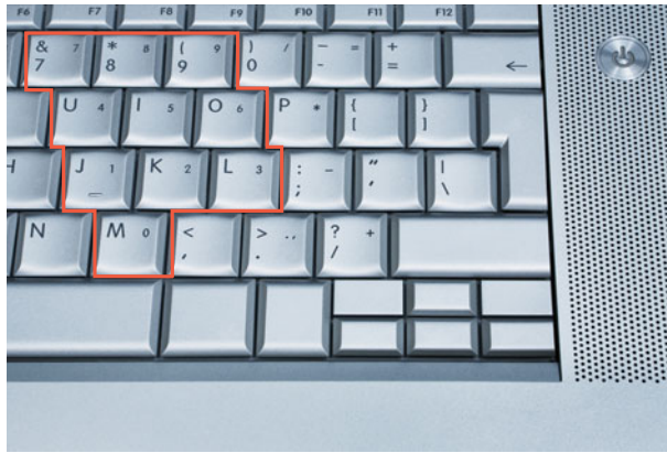
FIGURE 3.5 Some notebooks and netbooks use a series of adjacent keys that double as a number pad when a special function key is used.
