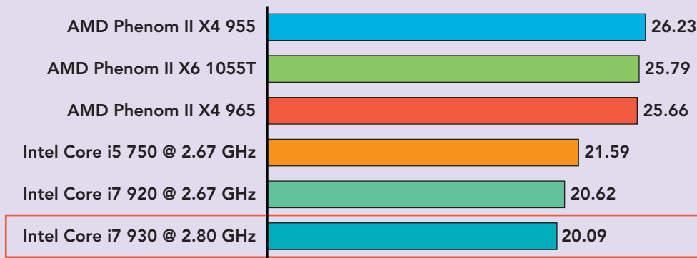
FIGURE 3D PassMark Software ( www.cpubenchmark.net ) provides benchmark test results for more than 300 CPU models and updates its results daily. The first graph shows the relative performance of the CPU compared to the 10 other common CPUs in terms of PassMark CPUmark. The second graph shows the value for money, in terms of the CPUmark per dollar.
