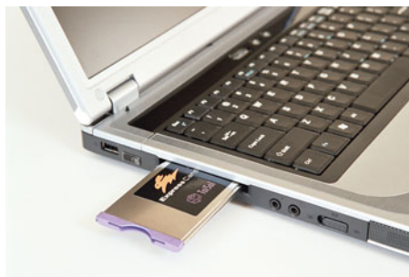
FIGURE 3.44 ExpressCards are about the size of a credit card and fit into ExpressCard slots, which are standard in most notebooks.
