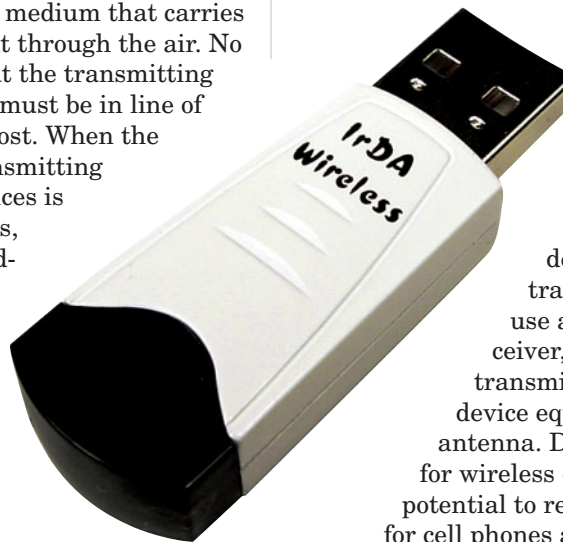
FIGURE 8.14 An IrDA port allows for wireless management of external devices such as a mouse, keyboard, phone, or PDA.
