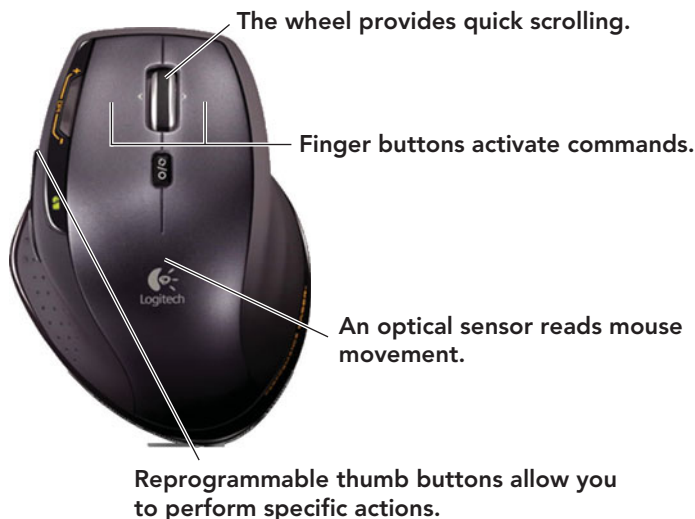
FIGURE 3.13 An optical mouse can be equipped with several thumb buttons that allow you to move between Web pages, zoom in on photos, or even reassign actions to them that meet your current needs.
