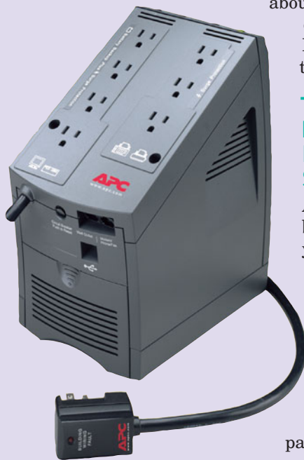
FIGURE 3H A UPS device can easily justify its purchase price by saving your data in an unexpected power outage.
