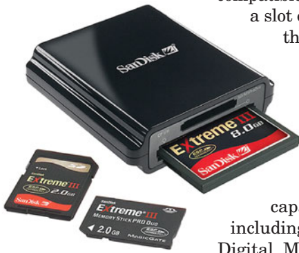
FIGURE 3.46 A flash memory reader can be used to transfer the contents of a memory card to your PC.
